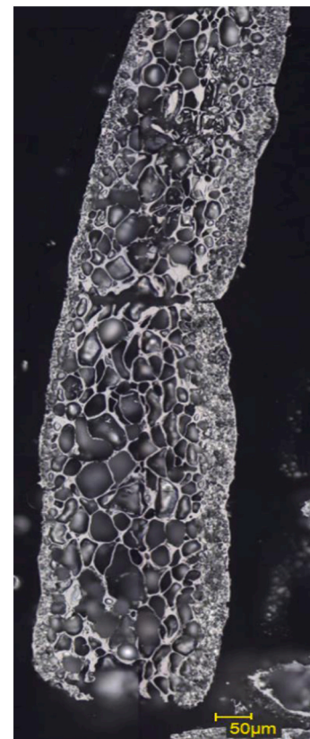
Fig. 9. A typical example of an inertinite maceral in biochar, captured in a white-light photomicrograph.
